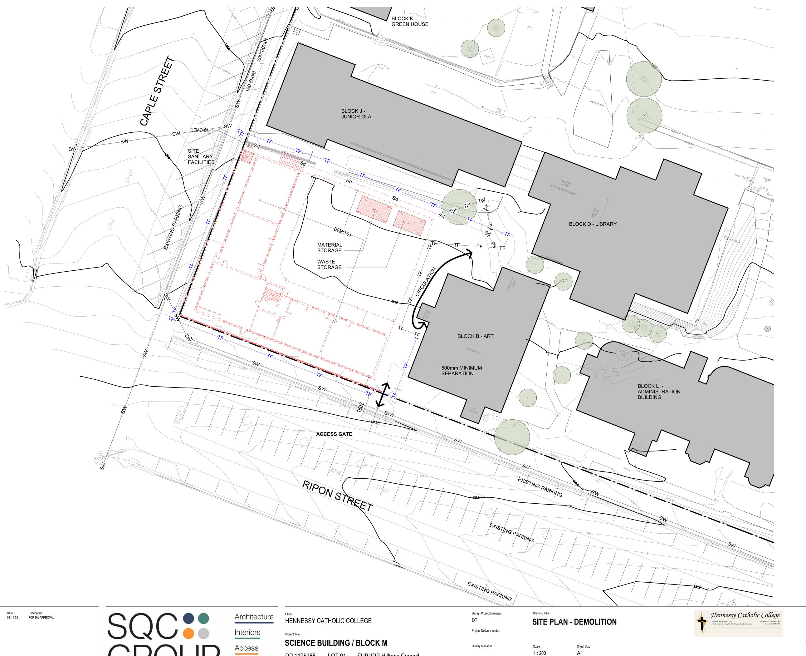
**LEGEND- DEMOLITION- SITE PLAN** ABC ANNOTATION ABBREVIATION. REFER KEYNOTES FOR DESCRIPTION EXISTING ELEMENTS DEMOLISHED ELEMENTS TREES TO BE RETAINED TREES TO BE REMOVED. REFER LANDSCAPE MANGEMENT & PROTECTION PLAN FOR MORE DETAILS TF-TF-TF TEMPORARY FENCE DURING CONSTRUCTION STw—STw STORM WATER SW—SW EXISTING STORM WATER Sd——Sd SEDIMENT CONTROL Tfp—Tfp TREE PROTECTION FENCE NOTES - DEMOLITIONS DESCRIPTION CODE
